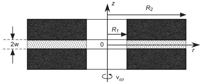
**Figure 3.** Configuration of the rotary shear experiments of Hirose and Shimamoto [2005]. The specimen consists of two coaxial thick-walled cylinders with inner and outer radii of  $R_1$  and  $R_2$ , respectively. One cylinder is fixed, while the other is rotated at an angular velocity  $\omega$ . The instantaneous thickness of the frictionally generated melt layer is  $2w$ .
