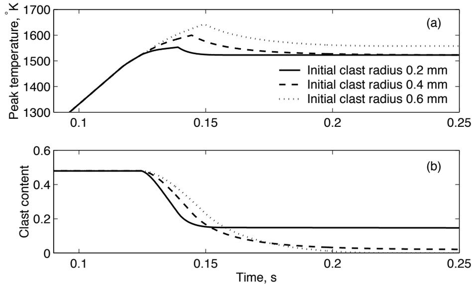
**Figure 5.** Evolution of (a) temperature and (b) content of the plagioclase (An45) clasts in a pseudotachylite of a tonalitic composition [Di Toro and Pennacchioni, 2004] due to fast fusion. Larger clasts give rise to a stronger temperature overshoot, and larger degrees of melting.
