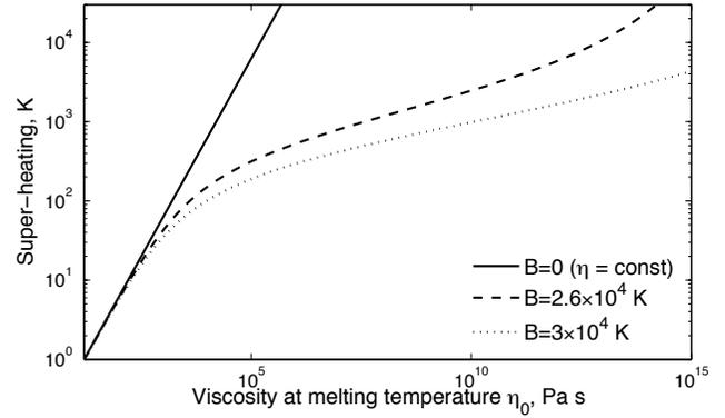
**Figure 2.** Maximum increases in the melt temperature at the center of the melt layer, for several values of the effective activation temperature  $B$ , and assuming slip velocity  $V_c = 1 \text{ m s}^{-1}$ , and thermal conductivity  $k = 2 \text{ W K}^{-1} \text{ m}^{-1}$ .
