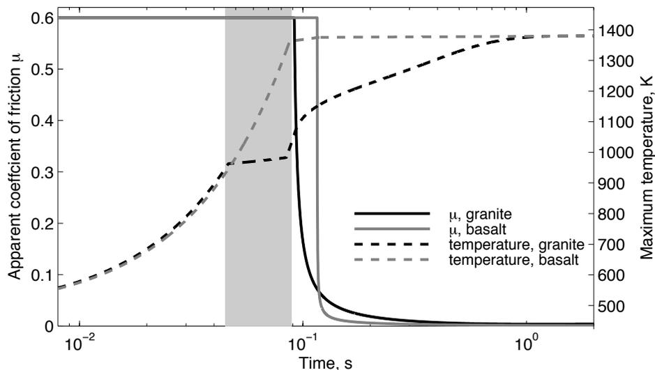
**Figure 6.** The effective coefficient of friction (solid lines) and the maximum temperature in the middle of the slip zone (dashed lines, right axis) for granitic and basaltic host rock compositions. The shaded area denotes an interval between the onset of melting, and the transition to the effectively viscous rheology in the model simulating slip in granite. This area represents a potential strengthening of the slip interface.
