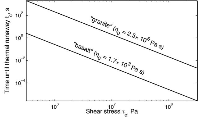
**Figure 1.** Characteristic evolution time between the onset of melting and the onset of thermal runaway for an adiabatic shear under a constant stress. “Basaltic” composition:  $A = 10^{-6}$  Pa s,  $B = 2.6 \times 10^4$  K,  $T_m = 1220$  K. “Granitic” composition:  $A = 10^{-7}$  Pa s,  $B = 3 \times 10^4$  K,  $T_m = 970$  K. Shown in parentheses is the corresponding melt viscosity at the onset of melting,  $\eta_0 = A \exp(B/T_m)$ .
